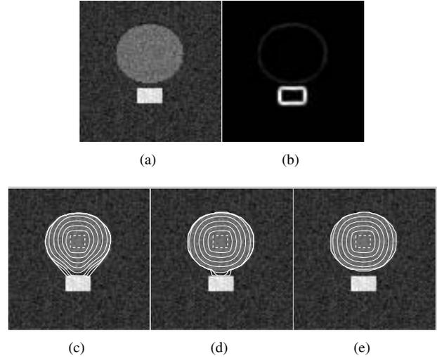
Figure 1. Performance of GVF, GGVF, and EPGVF. (a) The original image. (b) The edge map. (c) Evolution of the snake using GVF. (d) Evolution of the snake using GGVF. (e) Evolution of the snake using EPGVF
